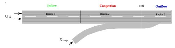
For the analysis, assume a macroscopic LWR model and a triangular fundamental diagram with the parameters
