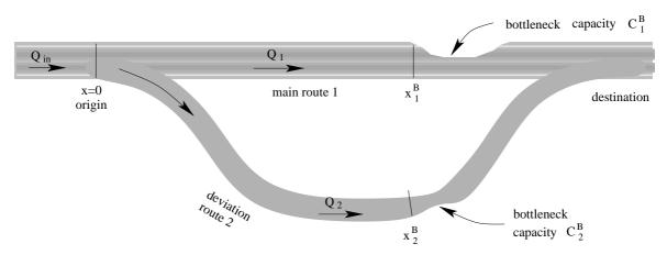
Furthermore, R1 and R2 have bottlenecks of capacities  $C_1^{\rm B}=4\,860\,{\rm veh/h}$  and  $C_2^{\rm B}=1\,080\,{\rm veh/h}$ , respectively that are located 14 km downstream of the merge (the precise position does not play a role, here). For simplicity, we assume no speed restrictions inside the bottlenecks. Use the LWR with a triangular funda,mental diagram for the following tasks.
